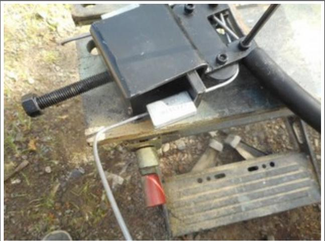
Once the tyre is firm on the rim prepare to join wire. Do not over tension. The machine is capable of enormous pressure. Back off tensioner 4 turns and slip the tyre off.
