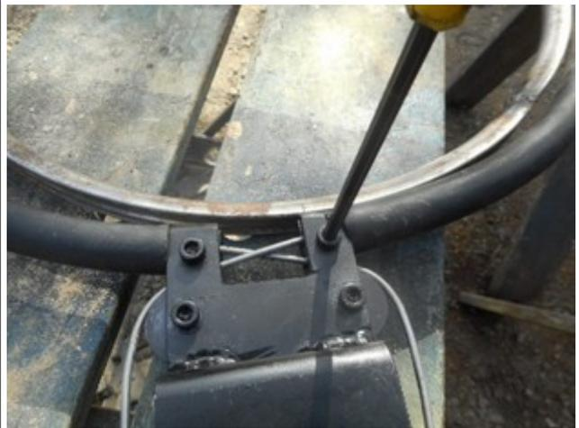
With the clamps locked lower the tension bar with the jacking screw.
