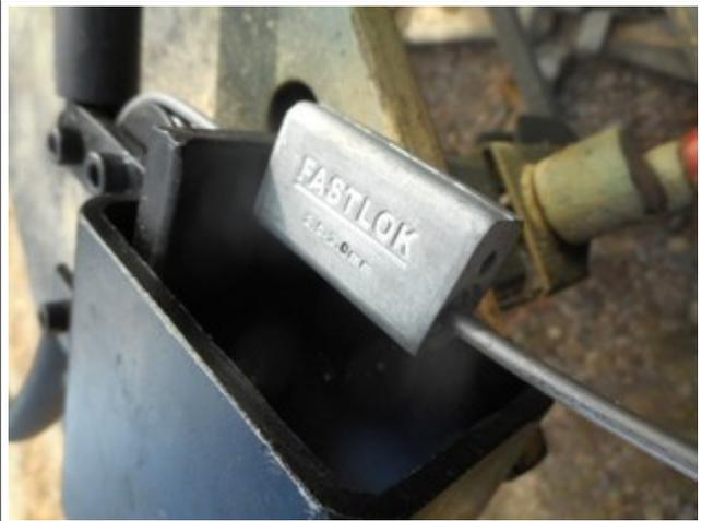
Tension the tyre with the jacking screw. At the limit lock the clamps as shown.
