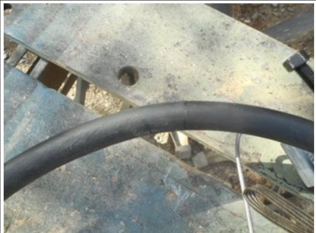
Roll/ snap the tyre on to the rim. Bigger wheels use tape or an assistant to get it back on.
