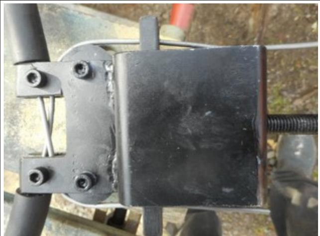
Fit the fastlok clamps. Small hole first over the wire.
