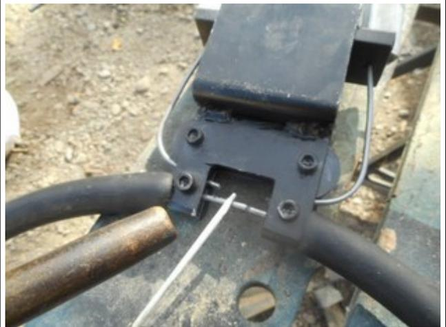
Minimise the gap between the wires.
