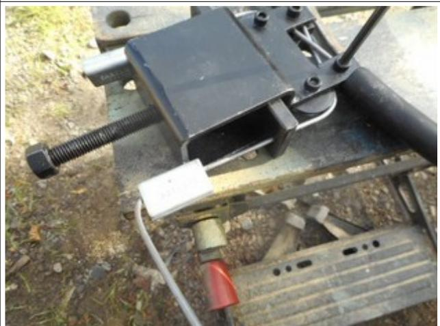
Push the fastlok clamp down and loosen the wire clamp. Use the jacking screw for another pull. Repeat as necessary.
